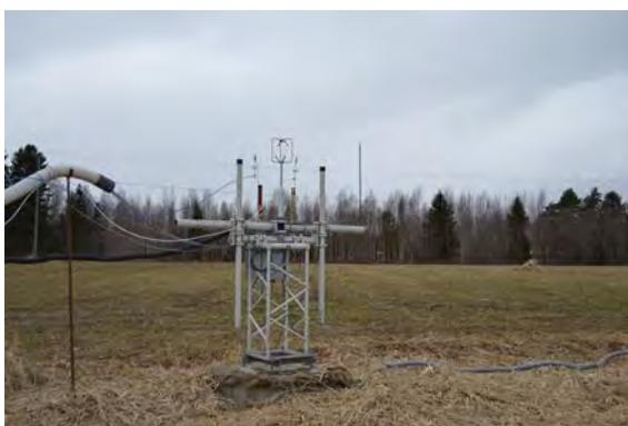
**FIGURE 1.** Eddy covariance measurements of CO<sub>2</sub> and N<sub>2</sub>O exchange from a perennial legume crop in Finland
