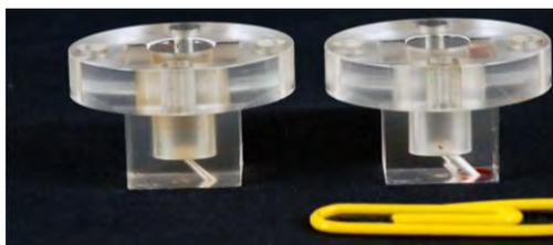
Figure 3: Diverging orifice (left) Sharp exit orifice (right)
