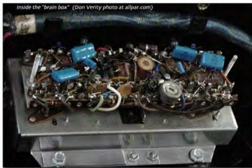
**FIGURE 4.** First Electrojector
