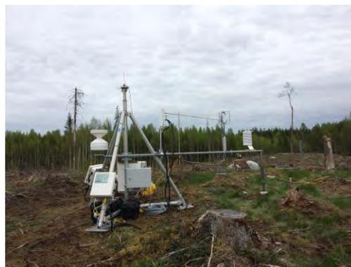
**FIGURE 2.** Eddy covariance measurements of CO<sub>2</sub> exchange from the floor of a clear-cut forest in Finland
