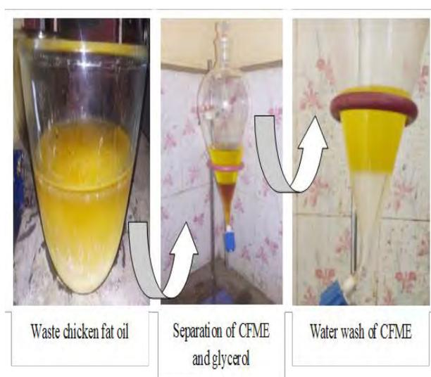
**FIGURE 1** Photograph of CFME production setup.
