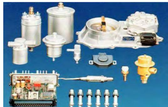
**FIGURE 6.** K Jetronic Components
