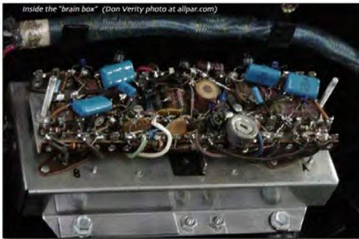
**FIGURE 4.** First Electrojector
