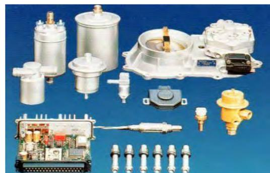
**FIGURE 6.** K Jetronic Components
