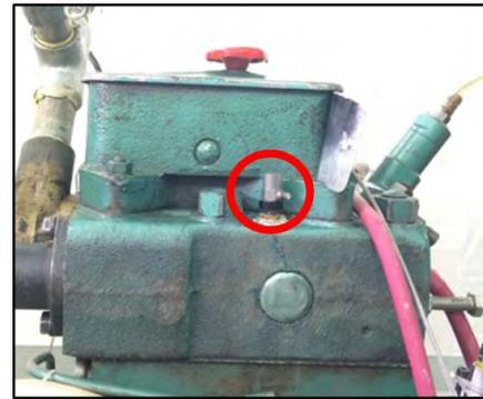
FIGURE 2. Accelerometer mounting position on the test engine.
