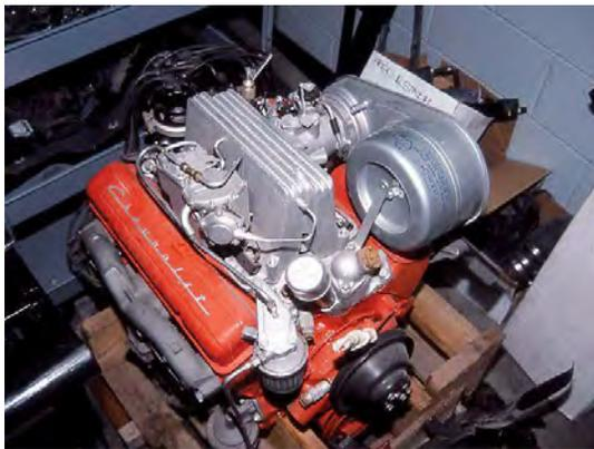
**FIGURE 3.** Chevrolet 1959 Corvette fuel injection
