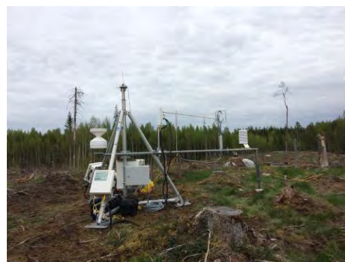
FIGURE 2. Eddy covariance measurements of CO 2 exchange from the floor of a clear-cut forest in Finland
