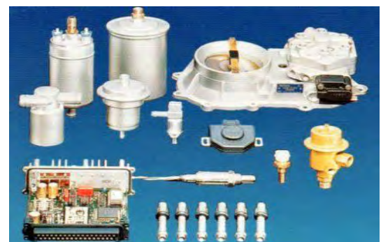
FIGURE 6. K Jetronic Components
