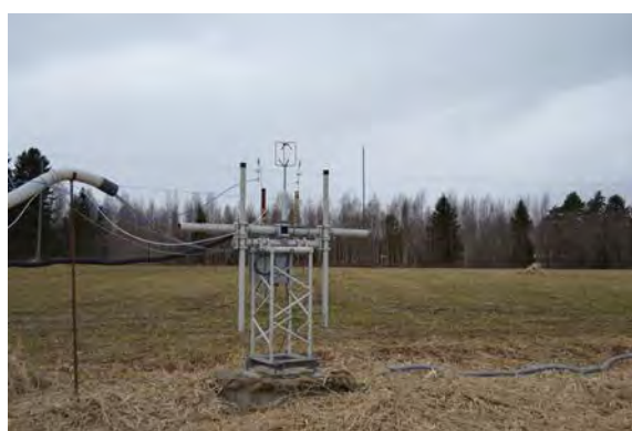
FIGURE 1. Eddy covariance measurements of CO 2 and N 2 O exchange from a perennial legume crop in Finland
