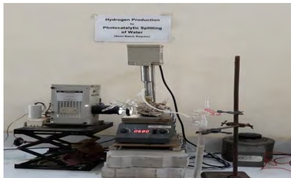
Figure1: Experimental set up for Hydrogen production by Photocatalytic splitting of water.
