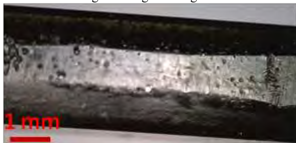
FIGURE 4. Worn surface of dual coated top piston ring
