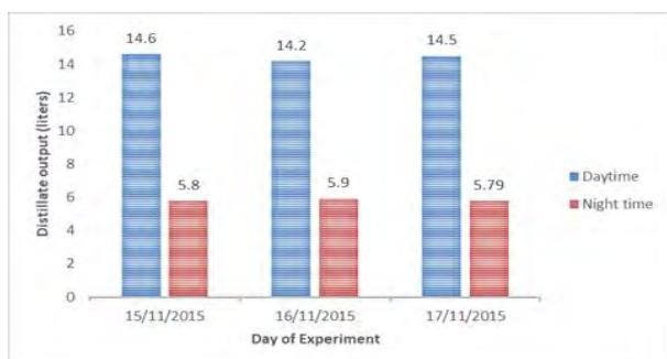
Fig.5. Day and night collection of distilled water
