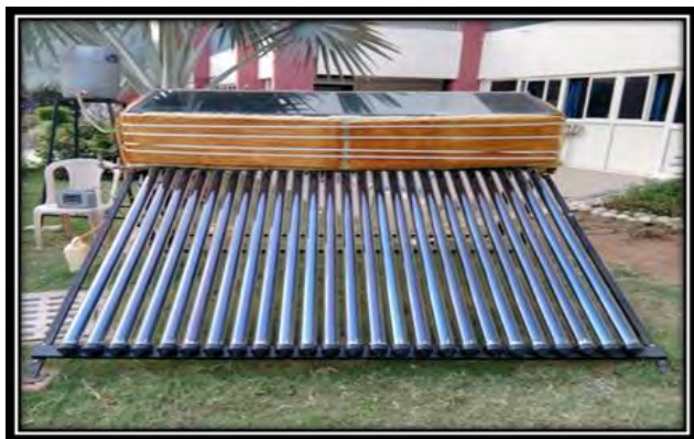
Fig.1 Experimental set up of triple effect solar still
